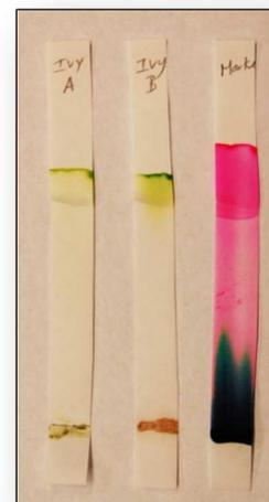
Chromatography is a technique that is used in laboratories when the different components within a solution of gas or liquid need to be identified. There are many different techniques for conducting chromatography, but all require that a liquid or gas moves through a material; the different chemicals within the solution move through the material at different speeds, causing them to separate out.
